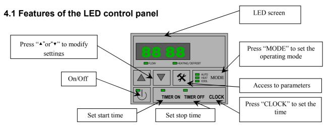
With the "On/Off" key "U", the heat pump is turned on or turned off (stand-by status). If the LED next to this key lights up, the heat pump is turned ON.
